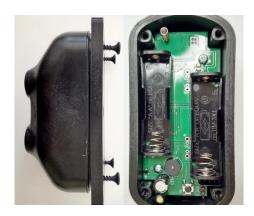
2. Attach the magnet to the sensor as shown in the picture (turn On/ Off ), you will hear the short beep 4 times.
