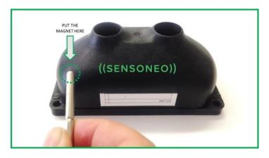
3. After initialization sensor starts to measure and logs into the network. Within 1 minute you should hear short beep 1 time. If the transmission is not complete you can hear short beep 2 times. In that case, you have to check whether the measurement was transferred to Sensoneo Waste Management System. Make sure you are in the coverage area of the network signal (LoRa or Sigfox).
